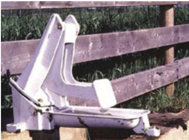
Nose pumps are operated by the actions of the animal
